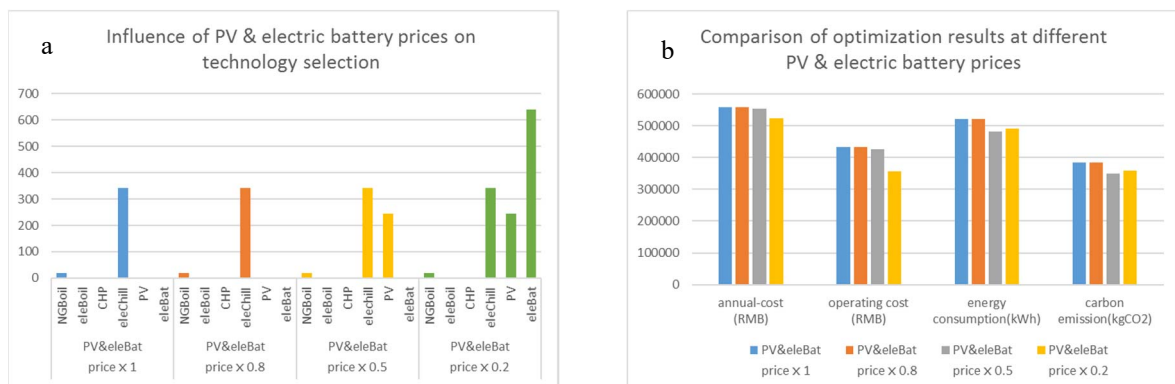
Fig. 4. Influence of PV and electric battery prices on optimization results. (a) Influence of PV and electric battery prices on technology selection; (b) Comparison of optimization results at different PV and electric battery prices
