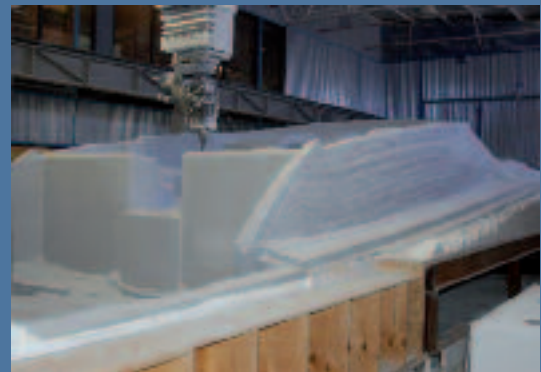
Parts up to fifty feet are machined with PowerMILL
