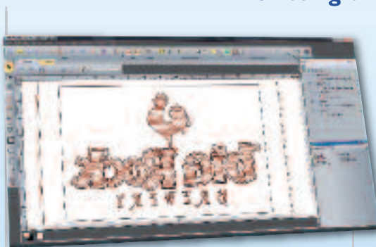
Using ArtCAM greatly reduced the amount of time needed to size, position and produce a mirror image of the logos
