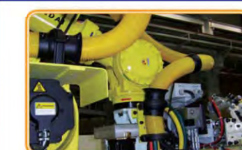
Spot Welding Robot
